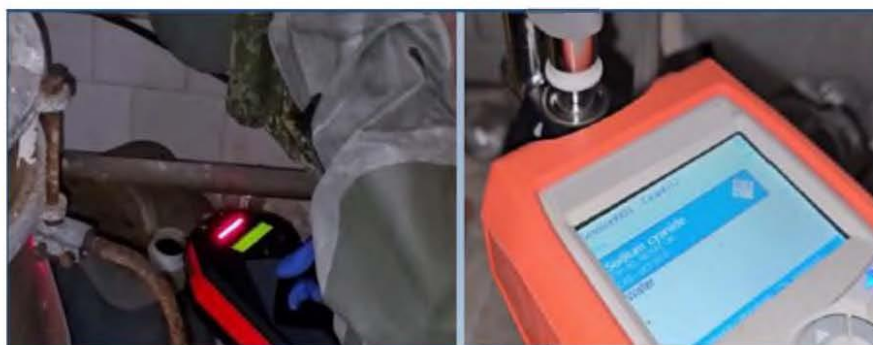
Rapid analysis sulfuric acid was detected in the canister and sodium cyanide was detected in the bulk container
