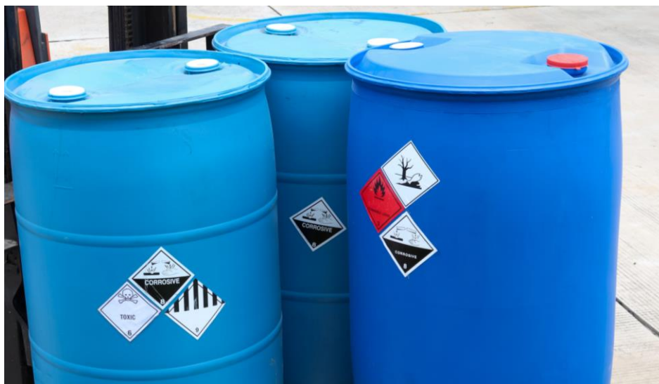
Figure 6. Example of packaging and labelling of hazardous chemicals.
