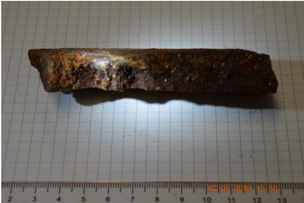
FIGURE 11: METAL FRAGMENT OF SAMPLE 03 SDS-01 SIDE VIEW SHOWING THICKNESS AND 90° ANGLED EDGES
