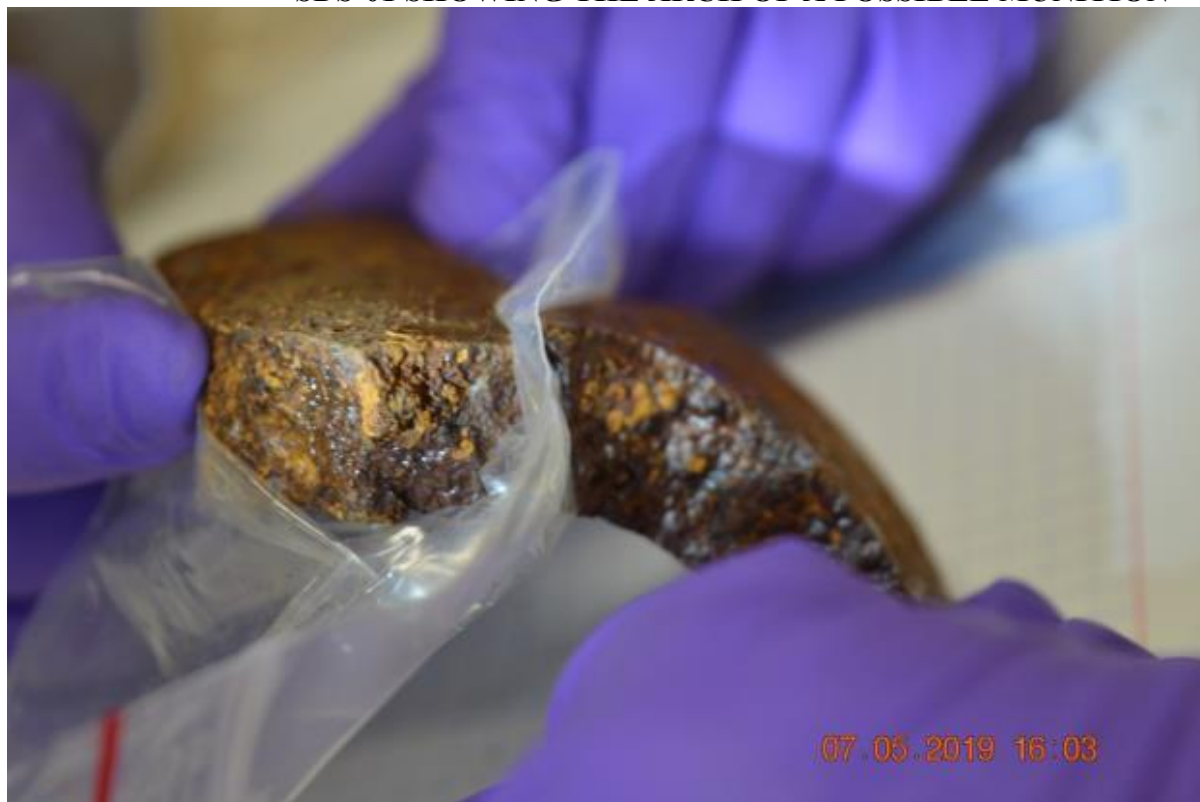
FIGURE 17: METAL FRAGMENT OF SAMPLE 03 SDS-01 AND SAMPLE 04 SDS-01 SHOWING THE ARCH OF A POSSIBLE MUNITION
