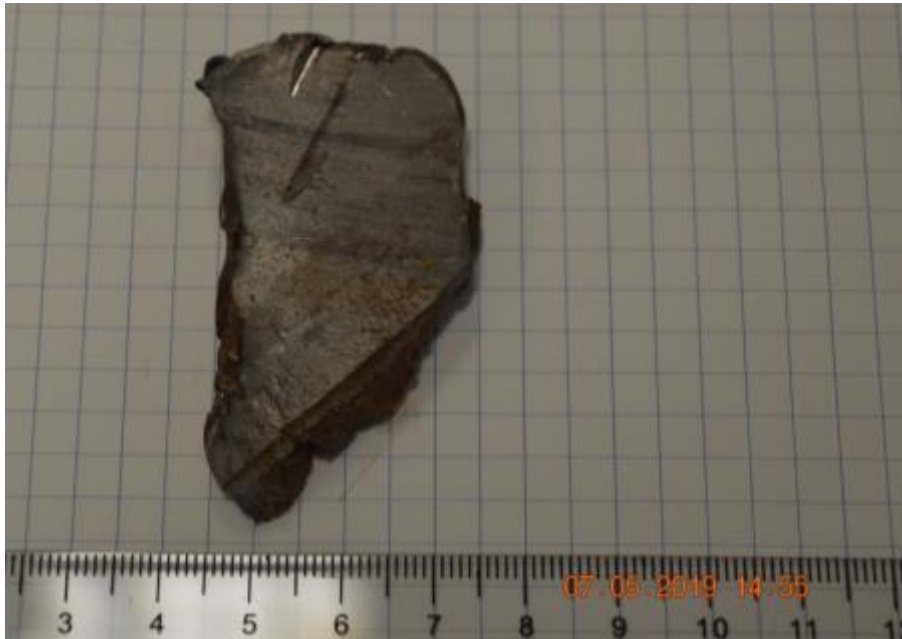
FIGURE 3: METAL FRAGMENT OF SAMPLE 08 SDS-01, SHOWING 45° DEGREE ANGLE EDGE
