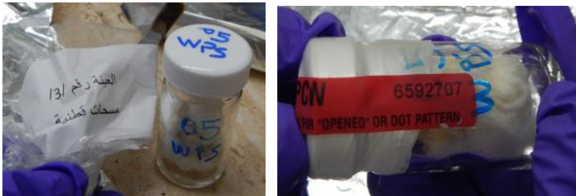
FIGURE 5: SAMPLE NO 05WPS – COTTON WIPE FROM GLASS OF ONE OF THE HOUSES NEAR THE IMPACT POINTS IN LOCATION 1
