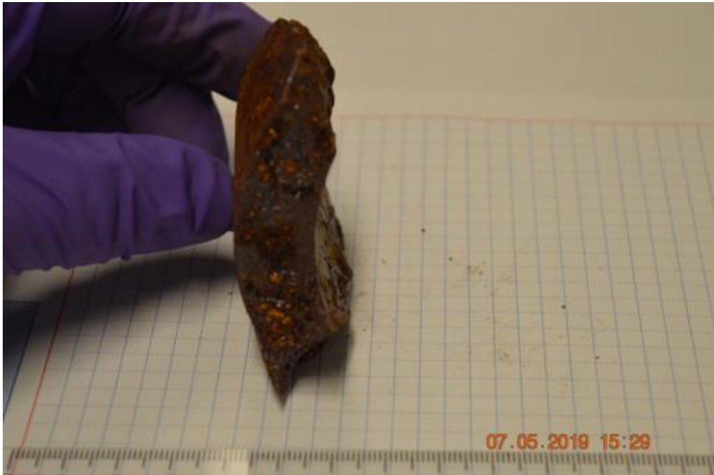
FIGURE 15: METAL FRAGMENT OF SAMPLE 04 SDS-01, SIDE VIEW SHOWING 90° ANGLED EDGES AND THICKNESS
