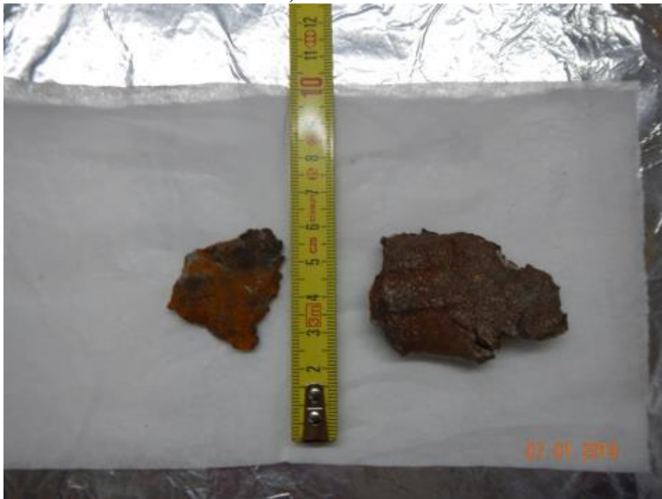
FIGURE 8: TWO METAL FRAGMENTS OF SAMPLE 09 SDS-01 OPPOSITE SIDE, SHOWING 45° DEGREE ANGLED EDGES
