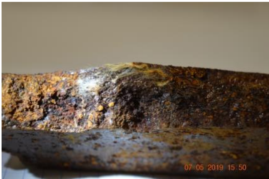
FIGURE 12: METAL FRAGMENT OF SAMPLE 03 SDS-01 OPPOSITE SIDE VIEW SHOWING THICKNESS AND 90° ANGLED EDGES
