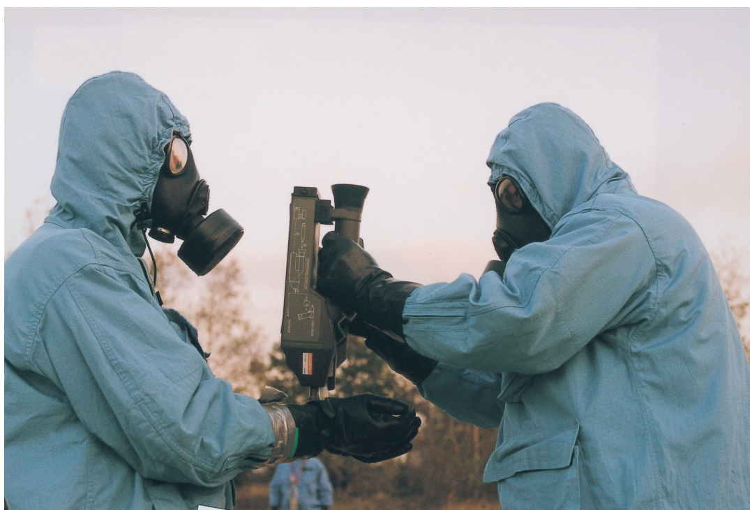
Inspectors testing a chemical agent monitor
